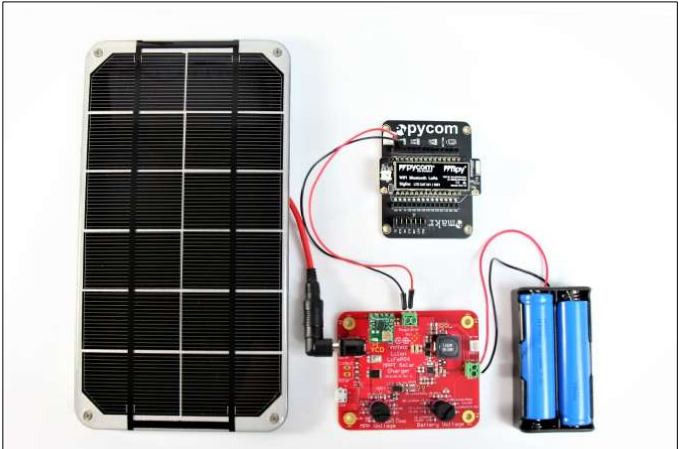
Figure 6: Example setup with panel, cells, and regulated output to microcontroller.
