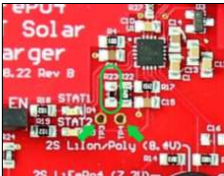
Figure 5: R23 embedded thermistor
