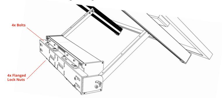
**Step 2 - Bracket Mount for V102 or V107 Batteries on BK108 Bracket -** With upper Bracket Bolt in place, attach battery to hook on bracket. Pass through second Bracket Bolt and tighten both bolts. <u>Wires on battery should face down</u>.
